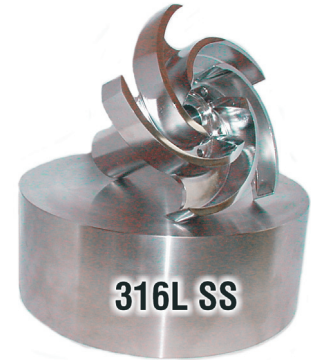
All Wet-end components are made from wrought 316SS, (UNS 31603) bar or flat stock with composition and manufacturing process controls that limit delta ferrite content to less than 5%.
