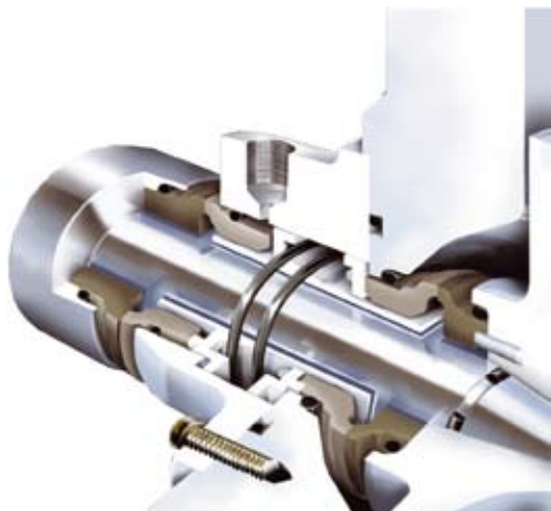
Double mechanical seal prepared for flushing or a steam barrier
