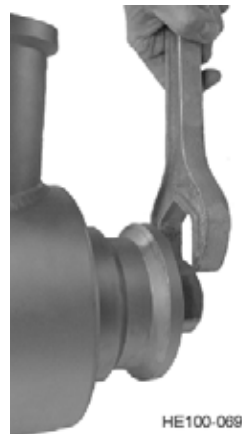
Figure 31 - Installation of Shaft Locknut
