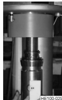
Figure 41 - Blade Alignment Tool Installed
