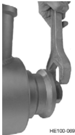
Figure 22 - Removal of Shaft Locknut
