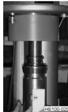
Figure 59 - Exposing Top Mechanical Seal
