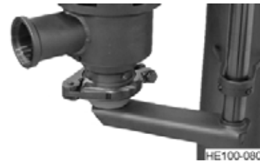
Figure 39 - Head Installed on Pin
