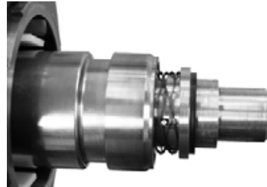
Figure 58 - Double Mechanical Seal Installed
