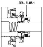
Drive end mechanical seal (Ceramic or Graphitar)
