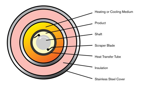
Votator's high efficiency and productivity results from a simple concept, heat or cool continuously moving product by providing a large heat transfer surface for a small amount of product in a confined space.
