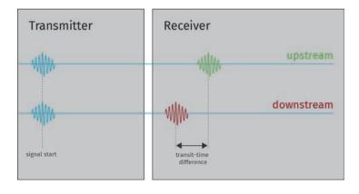
A typical transit time flow measurement system incorporates two piezo ceramics that act as both ultrasonic transmitter and receiver. The flow measurement is conducted by alternately transmitting and receiving an ultrasonic pulse between the two transducers and by measuring the transit time difference that it takes for the pulse to travel between them.
