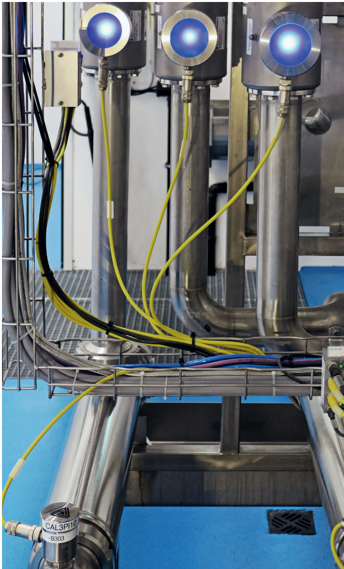
HH (bottom) and IZMAG (top) monitor process pressure and flow after the pumps in the three cleaning lines
