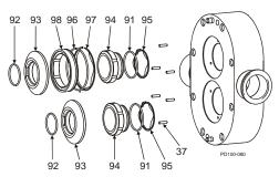
Figure 36 - Single (Bottom) and Double (Top) Mechanical Seal
