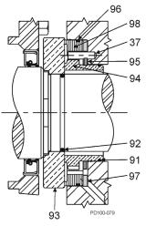
Figure 66 - Double Mechanical Seal
