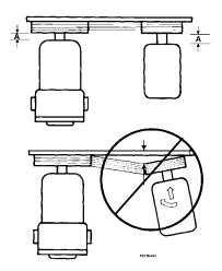
Figure 22 - Aligning Belt and Chain Drives
