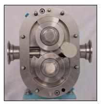
Figure 32 - Loosen Top Rotor
