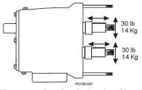
Figure 28 - Bearing Deflection Check
