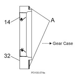
Figure 56 - Install Bearing Retainer
