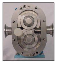
Figure 33 - Loosen Bottom Rotor
