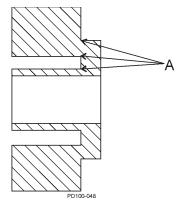
Figure 29 - Rotor Stress Points
