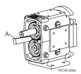
Figure 59 - Block Shaft Rotation
