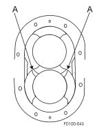
Figure 25 - Rotor to Rotor Tip Clearance
