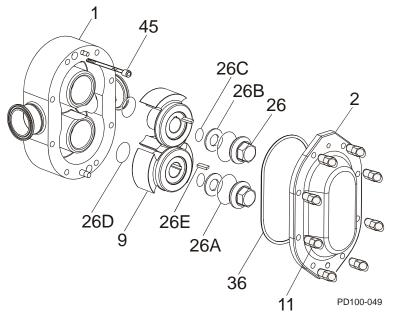
Figure 68 - Exploded View of Fluid Head
