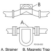
Figure 15 - Inline Strainers and Traps
