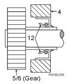
Figure 63 - Orientation of Oil Seal
