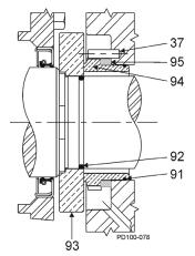
Figure 65 - Single Mechanical Seal
