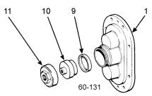
Figure 72 - Pneumatic Vented Cover
