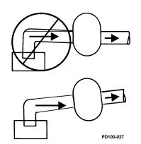
Figure 10 - Correct Piping to Prevent Inlet Air Pockets
