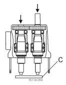
Figure 43 - Press Shafts from Gear Case
