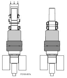
Figure 51 - Rear Tapered Roller Bearing
