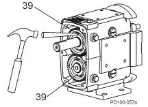
Figure 38 - Straighten Lock Tab on Lock Washers
