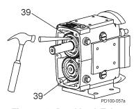
Figure 61 - Bend Lock Tab on Lock washers
