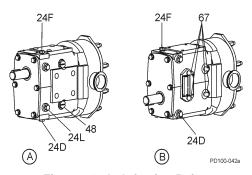
Figure 24 - Lubrication Points
