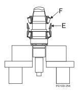
Figure 49 - Install Upper Cup & Upper Cone
