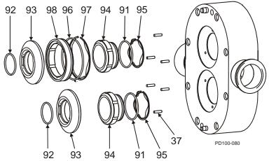
Figure 67 - Single (Bottom) and Double (Top) Mechanical Seal
