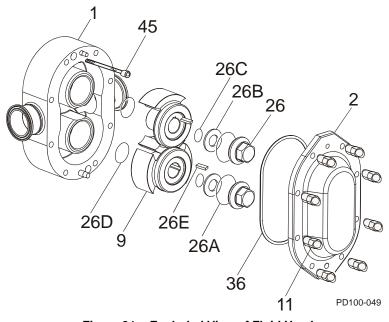
Figure 31 - Exploded View of Fluid Head
