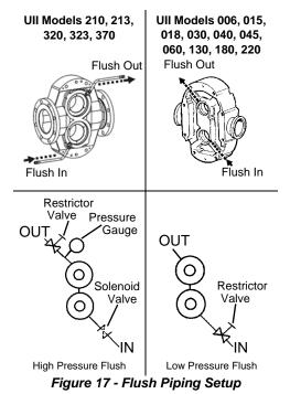
Pumps with double seals require flushing. The flush media (typically water) must be connected and flowing whenever pump is operated.
