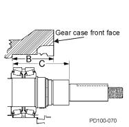
Figure 52 - Measure B and C
