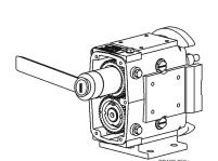
Figure 60 - Install Gear Locknuts
