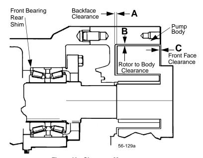
Figure 62 - Clearance Measurements
