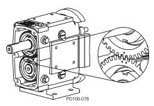
Figure 58 - Timing Gear Marks
