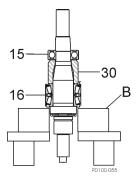
Figure 44 - Remove Bearings From Shaft
