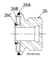
Figure 70 - Cross-Section View of Rotor Nut Assembly, as Assembled
