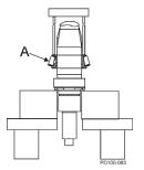
Figure 47 - Press Lower Cone onto Shaft
