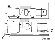
Figure 21 - Check Parallel Alignment
