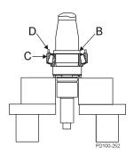
Figure 48 - Install Inner & Outer Spacer and Lower Cup
