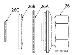
Figure 69 - Detail View of Rotor Nut Assembly
