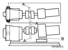
Figure 20 - Check Angular Alignment
