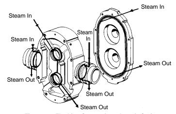
Figure 77 - Flushing Connection - Aseptic Series
