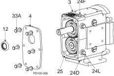
Figure 37 - Remove Gear Case Cover
