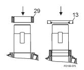
Figure 57 - Install Rear Seal
