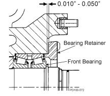
Figure 54 - Bearing Retainer Clearance
