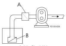
A. Inlet Check Valve B. Foot Check Valve
