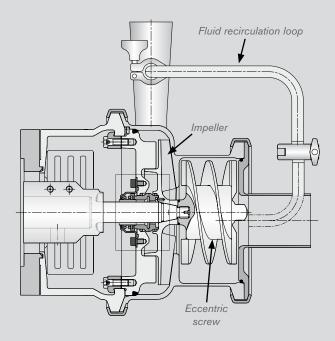
The APV Ws+ uses a unique design that combines the abilities of most liquid ring pumps with the efficiencies of the W+ centrifugal series. As a result customers can now handle entrained air and lift requirements with lower horsepower, less noise and at lower cost.
