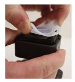
3. Lift actuator assembly from valve body.
