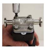
5. Install new diaphragm. Engage the threads of the diaphragm into the tube nut by rotating clockwise. Rotate the diaphragm until hard stop or heavy resistance is achieved and additional force does not significantly rotate the diaphragm into the compressor. See "PTFE Diaphragm Installation" instruction sheet for additional detail.
