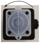
4. Unscrew the diaphragm from the compressor by turning counterclockwise..
