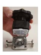
6. Back off (no more than 1/2 turn) until the bolt holes in diaphragm and the bonnet flange align. < 1/2 turn
