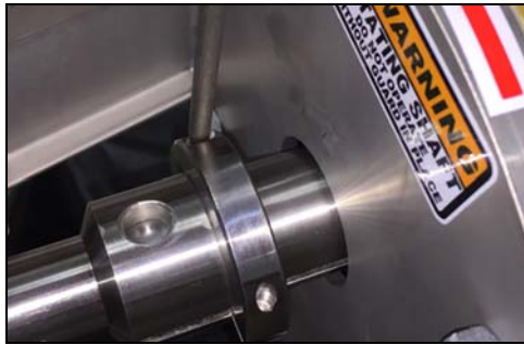
Figure 72 - Loosen shaft collar screws
