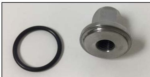
Figure 62 - Remove O-ring from impeller nut
