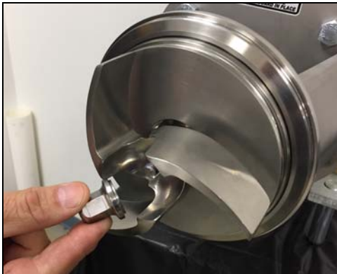
Figure 89 - Install impeller nut
