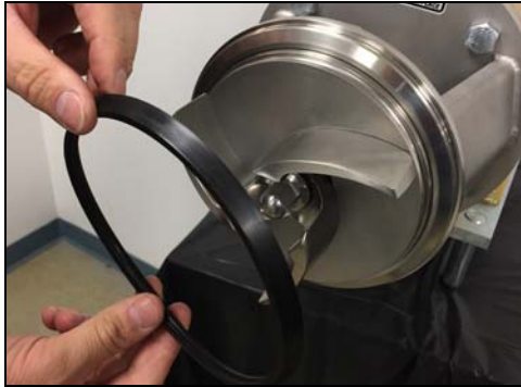
Figure 59 - Remove casing gasket
