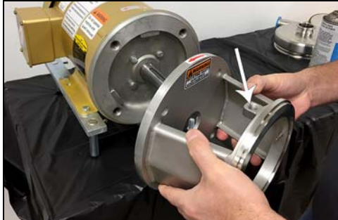
Figure 27 - Install motor adapter
