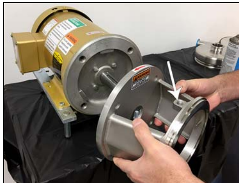
Figure 77 - Install motor adapter
