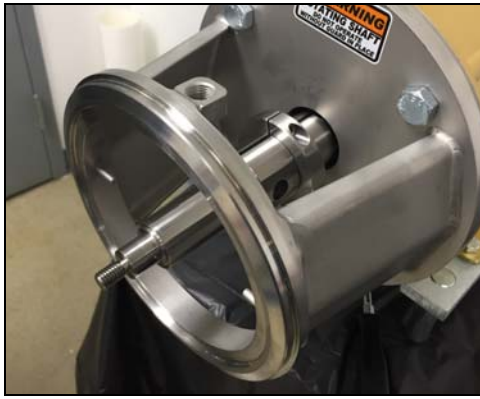
Figure 83 - Stub shaft on motor shaft
