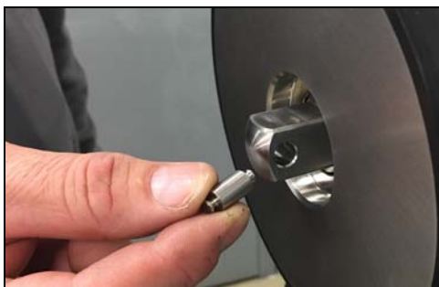
Figure 16 - Remove impeller pin
