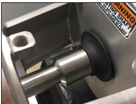
Figure 38 - Slide deflector onto shaft
