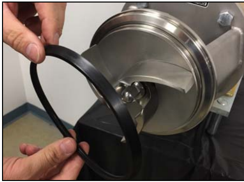
Figure 112 - Place casing gasket onto backplate
