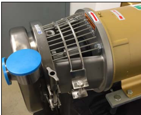
Figure 54 - Install guard assembly
