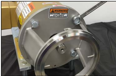
Figure 28 - Install motor adapter bolts
