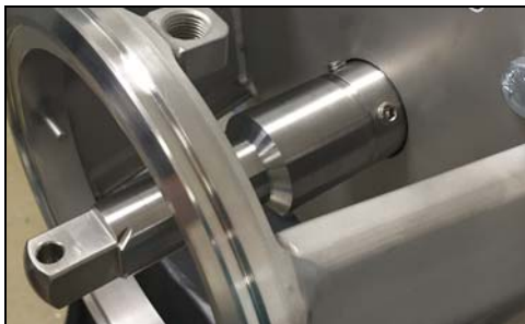
Figure 30 - Stub shaft on motor shaft
