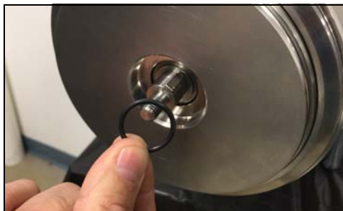
Figure 64 - Remove stub shaft O-ring
