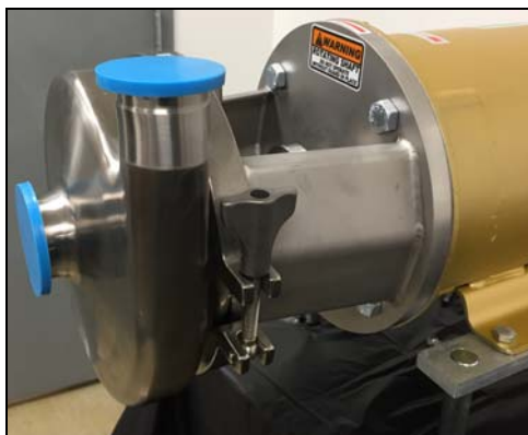
Figure 116 - Hand-tighten casing clamp
