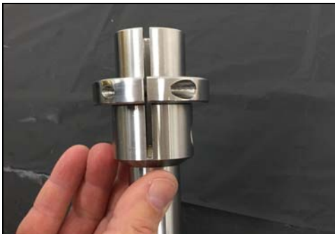
Figure 81 - Slide drive collar on stub shaft
