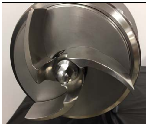
Figure 110 - Hand-tighten impeller nut
