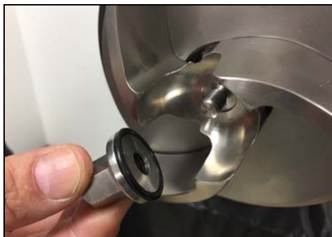
Figure 109 - Install impeller nut
