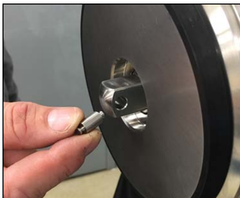
Figure 33 - Insert impeller retainer pin
