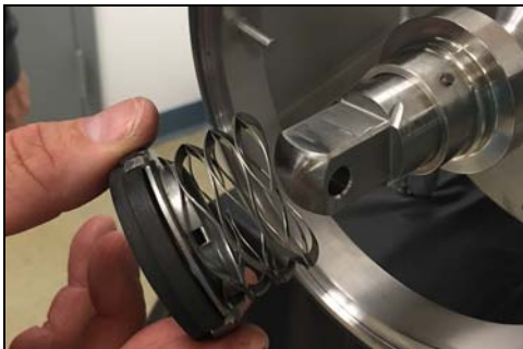
Figure 19 - Remove seal, O-ring, seal cup and spring
