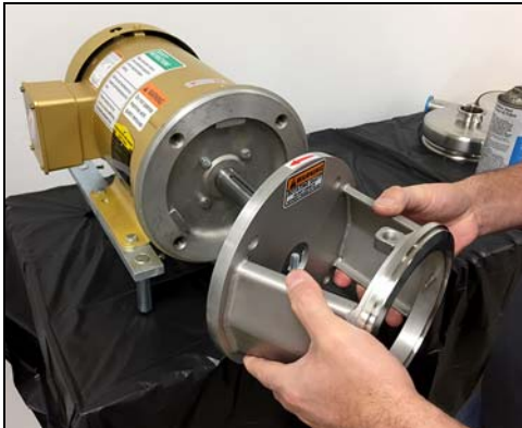
Figure 26 - Remove motor adapter
