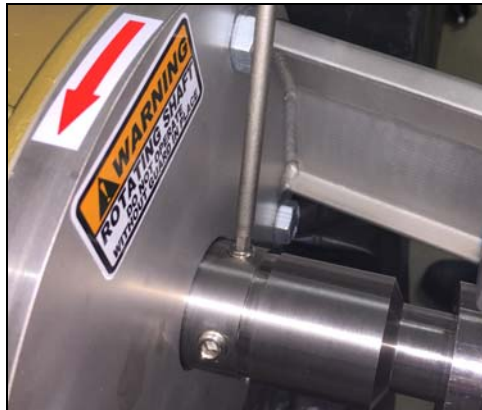
Figure 23 - Pin Impeller: Loosen setscrews
