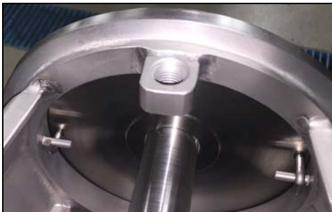
Figure 48 - Backplate pins engaged
