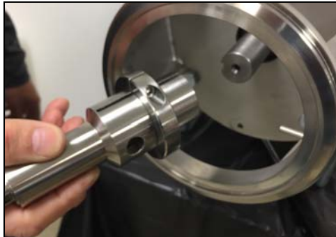
Figure 73 - Slide stub shaft off motor shaft
