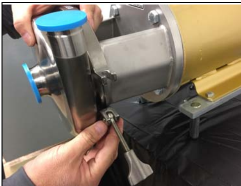
Figure 12 - Remove casing clamp
