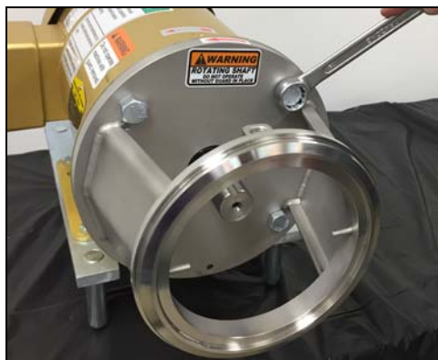
Figure 78 - Install motor adapter bolts
