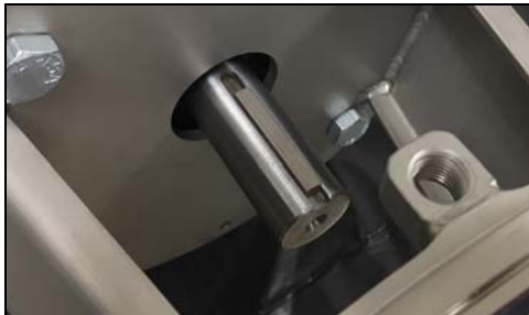
Figure 29 - Install key in motor shaft
