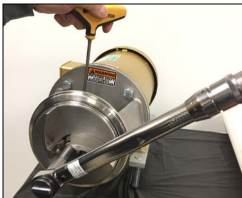
Figure 111 - Torque impeller nut
