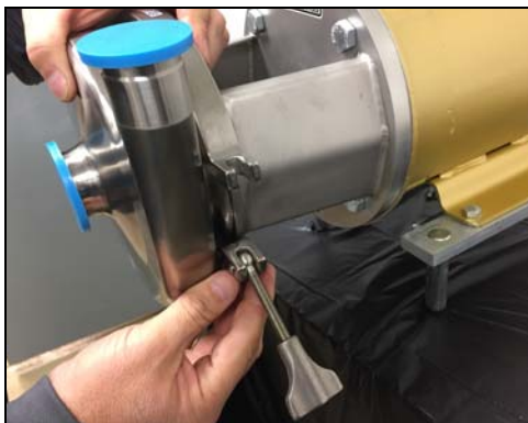
Figure 115 - Install casing clamp
