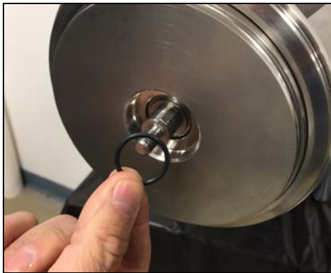
Figure 105 - Install stub shaft O-ring
