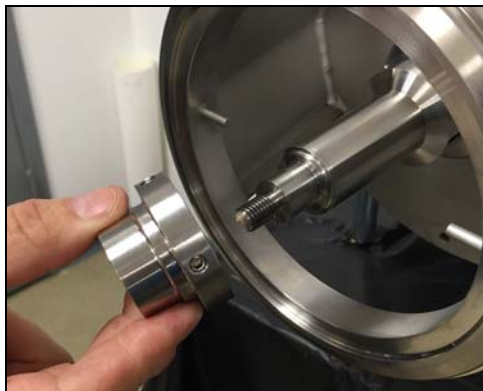
Figure 93 - Place drive collar on stub shaft
