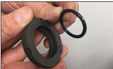
Figure 42 - Lubricate and install O-ring
