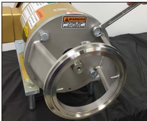
Figure 74 - Remove motor adapter bolts
