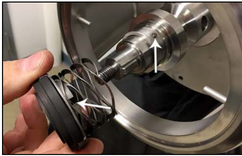
Figure 66 - Remove seal, cup, and spring
