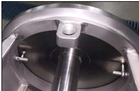
Figure 32 - Backplate pins engaged with adapter pins
