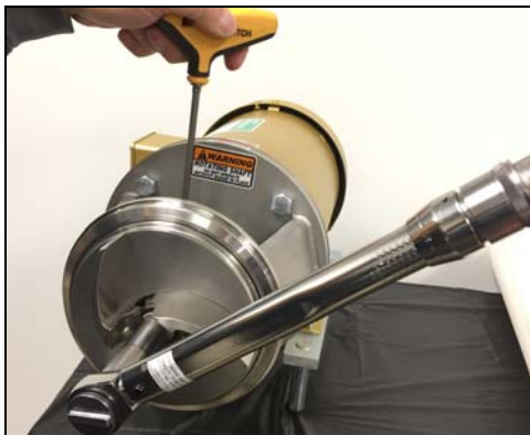
Figure 60 - Loosen impeller nut
