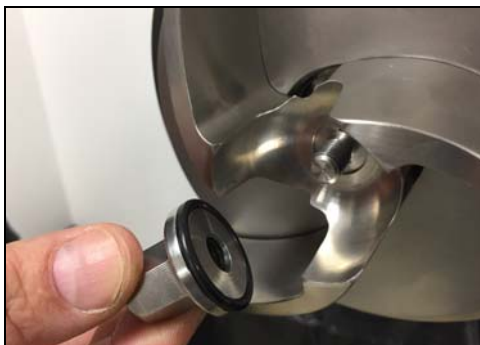
Figure 61 - Remove impeller nut
