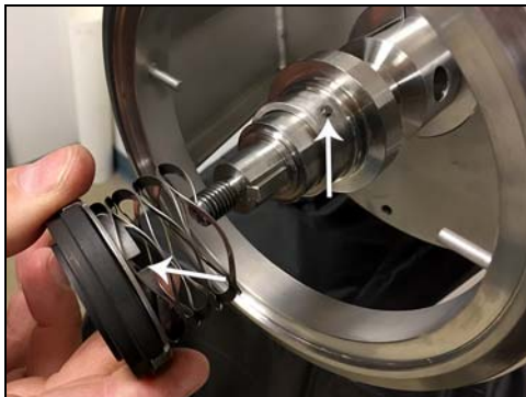
Figure 98 - Line up groove and pin
