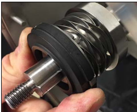
Figure 99 - Push seal on stub shaft
