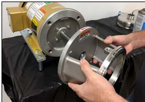
Figure 75 - Remove motor adapter
