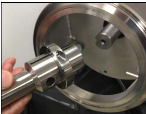
Figure 82 - Slide stub shaft on motor shaft
