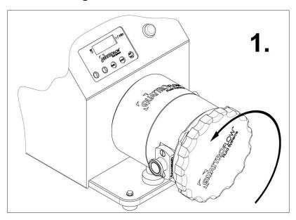
Unscrew the hand wheel (item 4) in rotational direction counter-clock wisely. 2-3 cycles are enough. It is not necessary to screw off the hand wheel completely.
