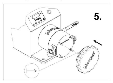
Assemble the whole subassembly (item 8) by placing the studs (item 6) into the provided holes and press it on. In addition to this, the mark on the bajonet-plate (item 2) should be visible. If the version without marking is present, the orientation of the subassembly (item8) will not matter.
