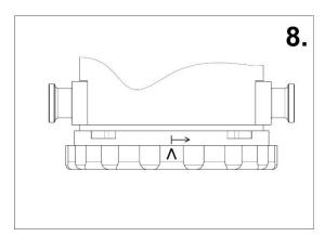
Fasten the hand wheel (item 4) by turning it clockwisely (figure 7). Turn the hand wheel until a noticeable drag appears. After that, the mark of the hand wheel must be turned at least to the mark of the bayonet-plate or beyond (figure 8). If the version without marking is present, the figure 7a must be observed for tightening.
