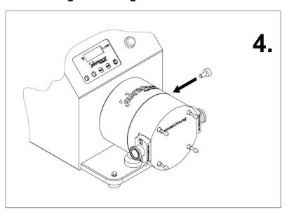
Tighten the locking screw with the help of a hex head wrench (Size 5mm).
