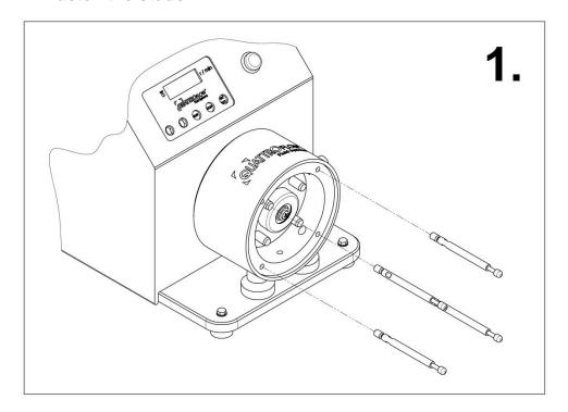
Fasten the studs (item 6) in the bearing-shell of the ring-drive-unit and tighten them with the help of an open-end spanner (A/F 5mm).
