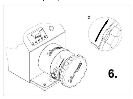
Fasten the bayonet-plate (item 2) by turning it clockwisely. The bayonet-closure snaps in after about 20° rotation-angle.
