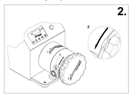
Loosen the bayonet-plate (item 2) in rotational direction counter-clock wisely. The bayonet-closure snaps out after about 20° rotation-angle.
