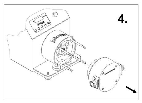
Pull the pump chamber off the studs (item 6).
