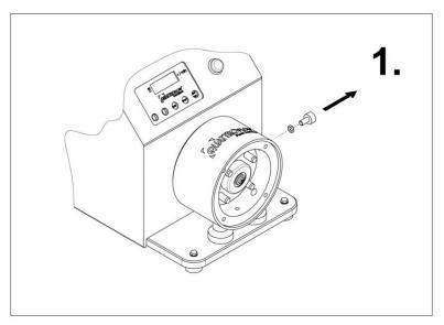
Loosen the locking screw with a hex head wrench (Size 5mm).
