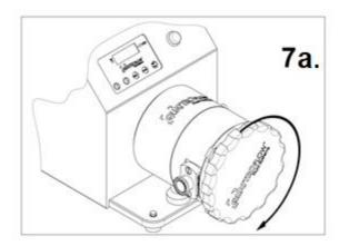
The hand wheel (item 4) must be turned so far until the rotational resistance decreases jerkily. Thereafter, it should not be further rotated until the next change of a new pump-chamber.
