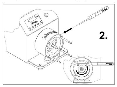
Align the cap of the shaft-bearing-cap-unit by the help of the adjusting stick (item 1).
