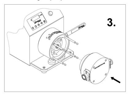
Assemble the pump chamber by the help of the studs (item 6). After that pull out the adjusting stick (item 1).
