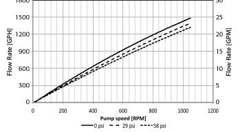
Depending on the selected motor/frequency drive combination, the motor frequency and the resulting pump speed might differ.
