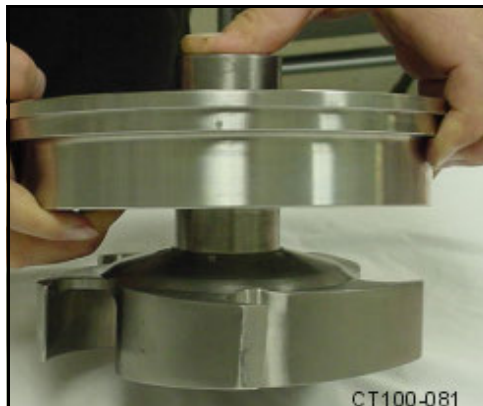
Figure 25 - Moving Rotary Seal Up the Shaft
