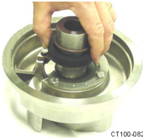
Figure 26 - Push Rotary Seal Down
